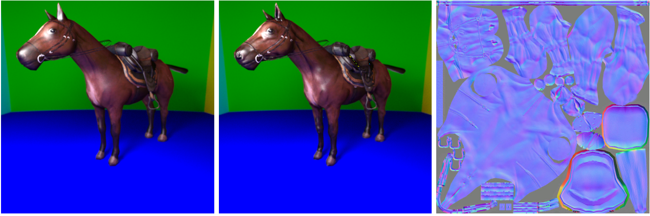
Figure 2.41: Horse model without (left) and with (middle) normal mapping ; the normal map of the body is illustrated on the right. The code is about 850 lines and runs in 1min 12s (left) or 1min 15sec (right) using 1000spp and 5 bounces. The mesh has only 5333 polygons, but normal mapping makes it look more complex. The mesh can be downloaded here: http://www.cadnav.com/3d-models/model-46223.html . It has been rotated like the cat, scaled by 0.15 and translated by (10, -10, 0). The order of the textures to be loaded (since there is no .mtl file) is: body2.d.tga , gear.d.tga , body2.d.tga , gear.d.tga , body2.d.tga
