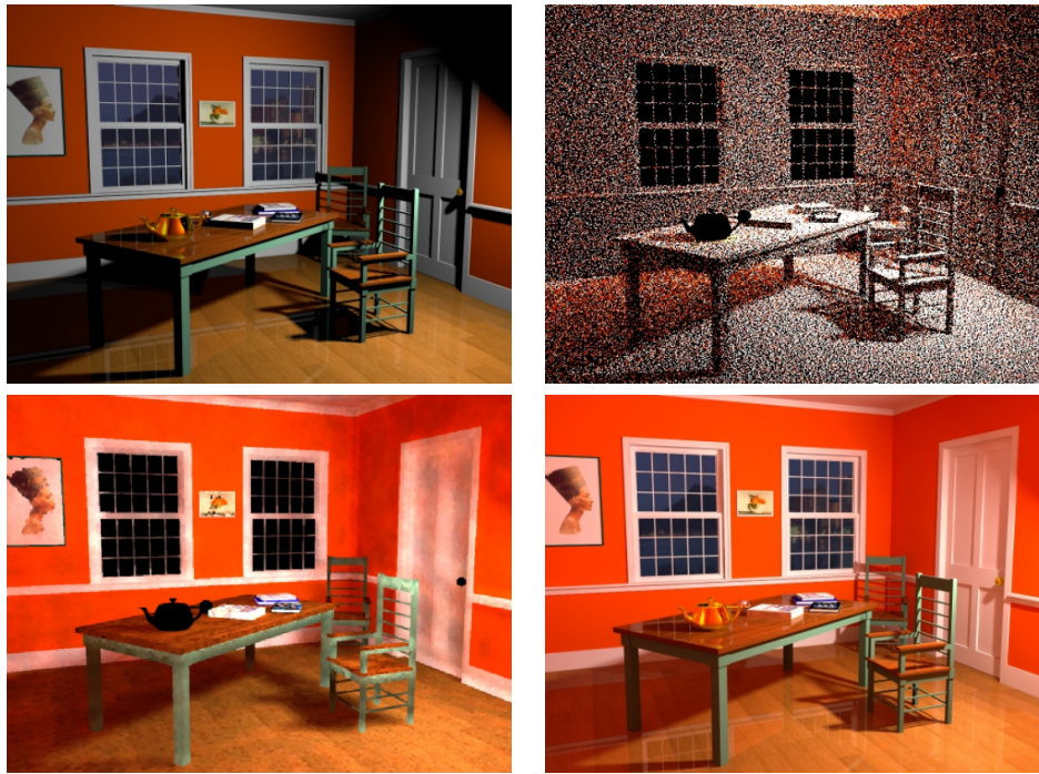
Figure 2.46: Interior scene: (a) Traditional ray tracing. (b) Photon map. (c) Precomputed radiance estimates at 1/4 of the photon positions. (d) Complete image with direct illumination, specular reflection, and soft indirect illumination. Fig. 5.2 of the SIGGRAPH 2002 course “A Practical Guide to Global Illumination using Photon Mapping”.
