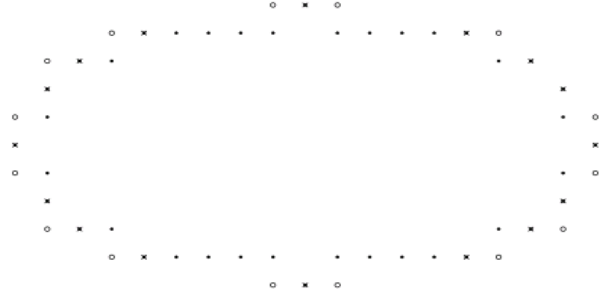
Figure 3: Given a digital curve (dots), S (crosses) and T (circles) are computed in linear time [3]
