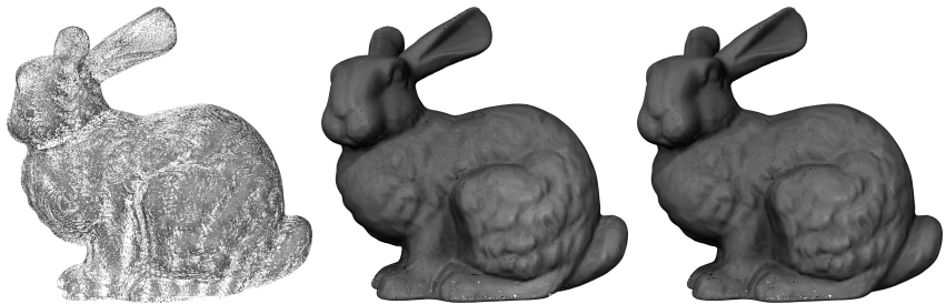
Figure: Reconstructing the Stanford Bunny point cloud, with a single radius (0.0003), two radii (0.0003; 0.0005) and three radii (0.0003; 0.0005; 0.002).
