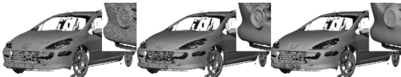
Figure 11. Denoising of a data set acquired with a range laser scanner (left: original, middle: our denoising, right: bilateral filter).
