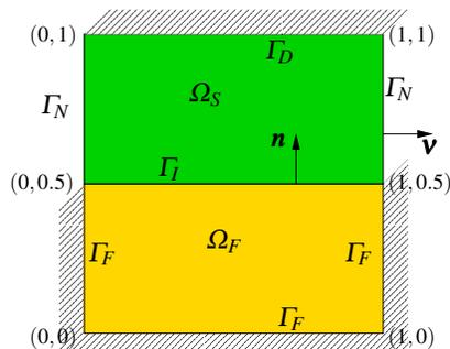
FIG. 2. Problem with analytical solution: sketch of the domains.
