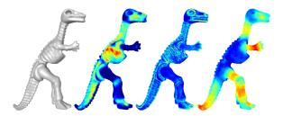
**Figure 1:** Some examples of vertex attributes, for the Dyno mesh (42K vertices). From left to right: Original model, roughness, local curvature (geodesic radius = 1% of the bounding box max length), global curvature (geodesic radius = 5%). The values are represented from blue (low) to red (high).
