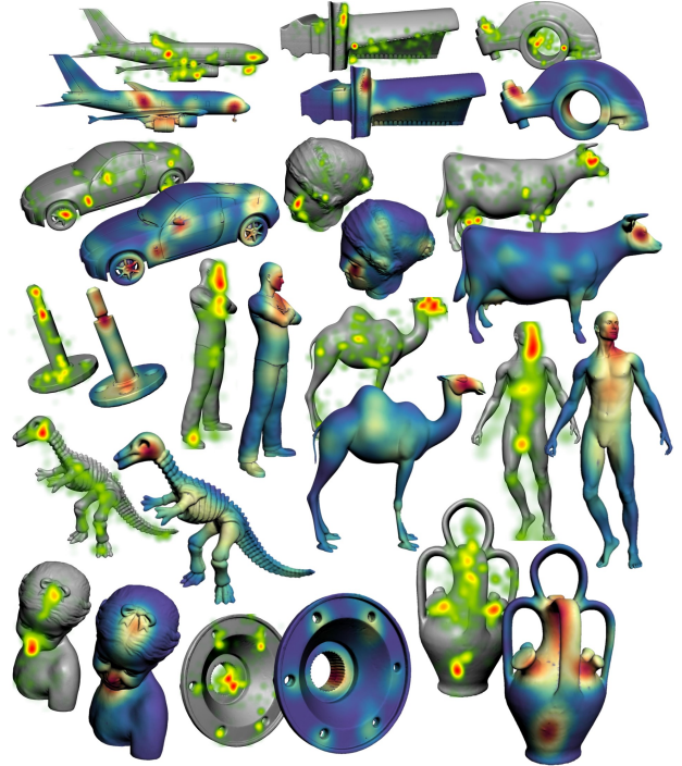
Figure 10: 2D heat maps and 3D mesh fixation maps for several objects. From left to right and top to bottom: A380, Turbine, RockerArm, Car, Igea, Cow, Meca, James, Camel, Michael3, Dinosaur, Bimba, Carter and Vase.
