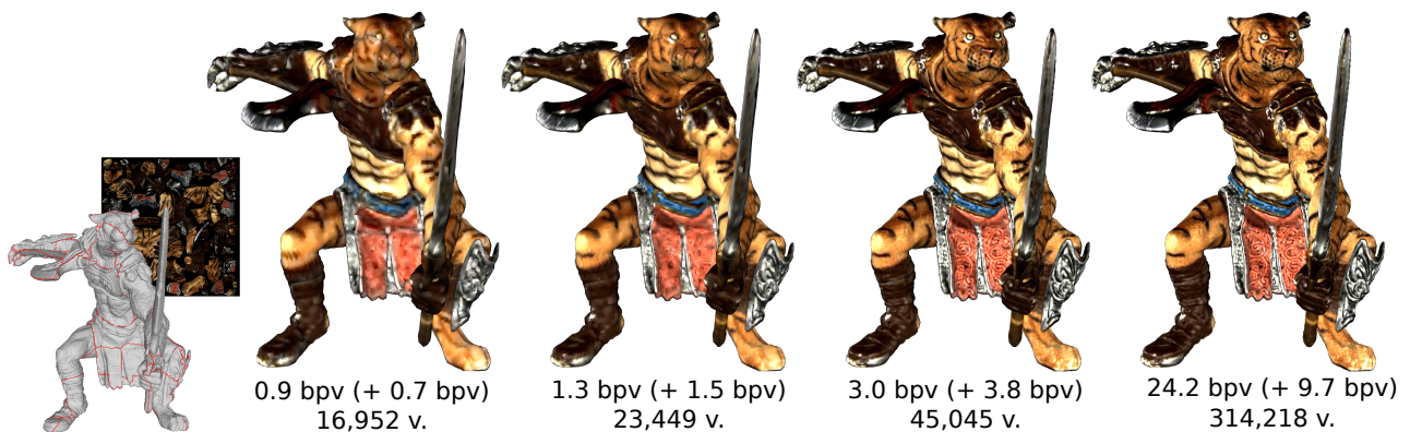
Figure 1: Progressive decomposition of the Tiger Fighter model (314,218 vertices). For each level of detail, we present the total size of the decoded data for the mesh elements (geometry, connectivity, texture coordinates) and for the texture image (in parentheses) in bit per vertex, as well as the number of vertices. Texture seams are illustrated in red.
