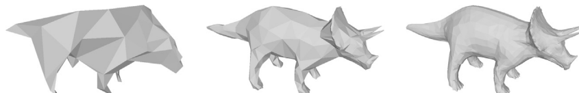
Fig. 8. Results obtained with the progressive compression algorithm [17] on our triceratops 567-remeshed model. From left to right, coarsest, medium and highest mesh resolutions are presented.
