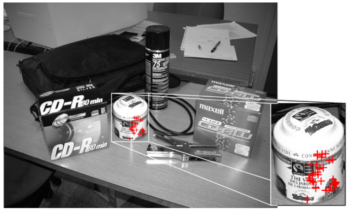
Figure 2: Result of recognition over a cluttered image. Red crosses indicates the final assumed positions of the keypoints defined in the model. Despite the fact that the box is viewed from a different angle than in the model, the recognition achieves a nearly exact extrapolation of the model pose. The whole process spends about 1s for keypoints extraction and 0.01s for recognition.
