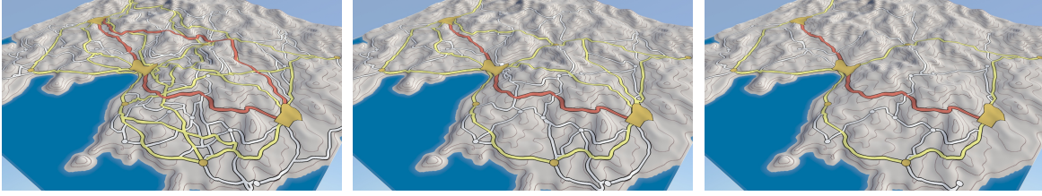
Figure 14: Different road networks connecting 3 cities, 6 towns and 16 villages: dense \gamma = 1.2 (left), average \gamma = 2.0 (middle) and sparse \gamma = 8.0 (right). The networks were created on a 128 \times 128 \text{ km}^2 terrain discretized into 256 \times 256 resolution.
