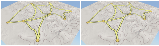
Figure 16: Simplification process showing an initial network (left) and the resulting simplified network (right).
