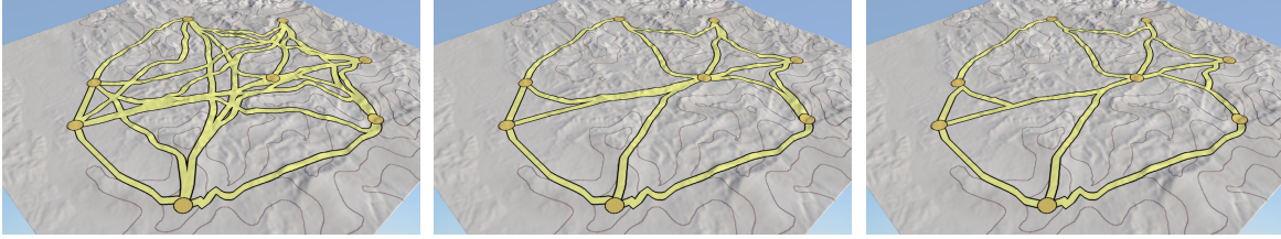
Figure 6: Overview of the road network generation algorithm for a given road type: the complete graph connecting cities (left), the generated proximity graph (center) and the final road network obtained after merging the close parts of the different road paths (right).
