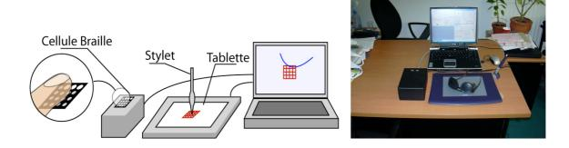
Fig. 5. Tactos system including the stylus and the graphic tablet, the computer and the Tactos software, the braille piezoelectric cells matrix
