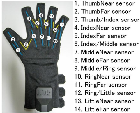
Figure 2. Name of each data glove sensor
