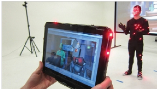
PhaseSpace's active LED systems now work with easier-to-wear, thumb-sized controllers and can include accelerometers.
