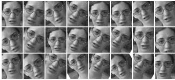
Figure 4: Examples of training images created by manually misaligning the face (top left: well-aligned face image).
