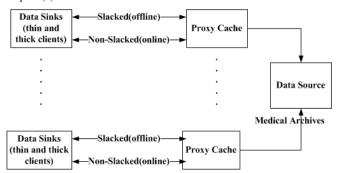
Figure 4. A High-Level System Architecture for the Settings of the Complex/Multi-context Prefetching
