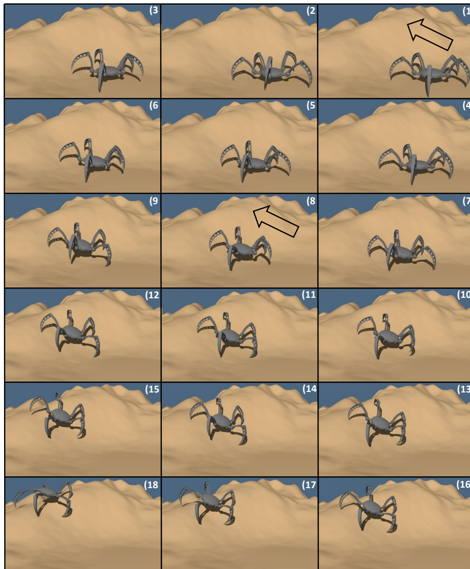
Figure 3.37: A 5-legged robot going uphill.
