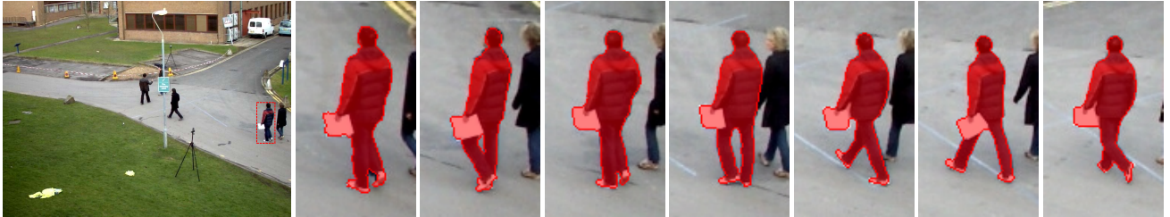
Fig. 3. Local matching-based probability estimation applied on a PETS 2009 crowd sequence (with narrow perception)
