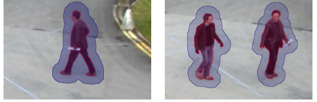
Fig. 1. Background perceived by target region (outlined with red curve) is limited within narrow band (outlined with blue curve). Other moving people do not intervene in the background representation of target
