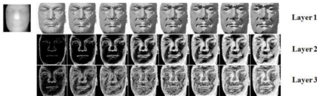
Fig. 1. A set of eLBP based depth maps of a facial range image with 8 neighboring points ( P = 8 ), different radius value R from 1 to 8 (from left to right), and 3 layers ( L = 3 )
