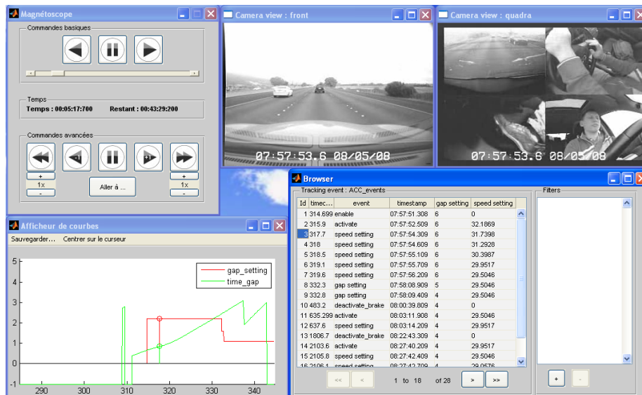
Figure 4.1: An example of a synchronised visualisation possible with BIND. From left to right and top to bottom: a controller, the front video, the quadravision video, a display of curves and a list of events. Everything is synchronised.
