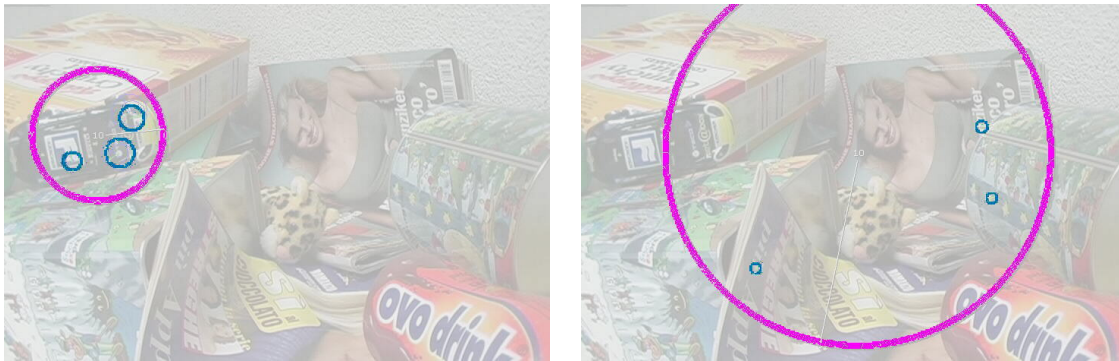
Figure 3.6: Noise affects more clusters of hypothesis having a large support (outer purple circle), as their surface absorbs more false aggregates (small blue circles). Left: a positive detection (the toy car); right: a negative detection for the same object.
