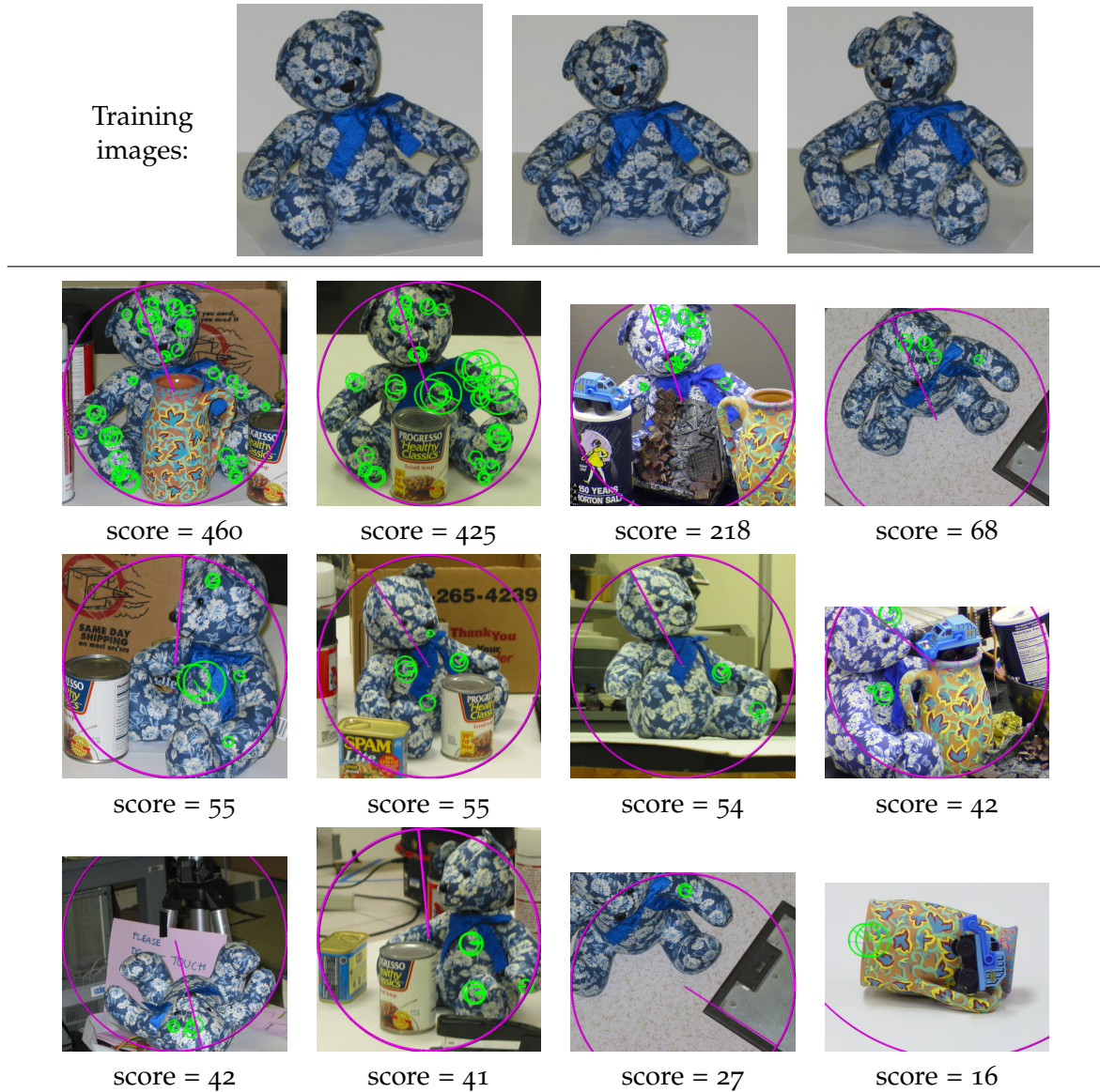
Figure 4.14: Illustration of the robustness of our method to viewpoint change. (Top) The three training images of the teddy bear used to train the lattice (orientation is defined vertically for the three images, n_{term} = 90 ). (Bottom) Top scoring detections on the Rothganger dataset using the lattice thus created (small green circles indicate the position of detected aggregates, large purple circles indicate the hypothesized object location and pose). Our method shows an impressive tolerance to viewpoint change (the first negative detection comes with a score of 16, after the 11 th positive image). The quality of the 10 th detection is questionable due to bounding box misplacement. The next detections (with scores inferior to 16) are all true negatives.
