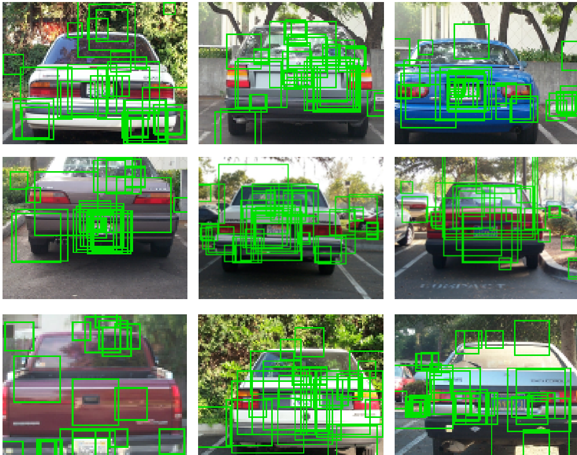
Figure 6.7: Sample detections on the “car-rears” dataset (only the highest-ranked window per image is shown). Aggregates used by the classifier to rank the window are highlighted in green squares. As can be observed, most squares are positioned on object parts rather than on the background, demonstrating that our lattice construction procedure is well able to learn discriminative aggregates.
