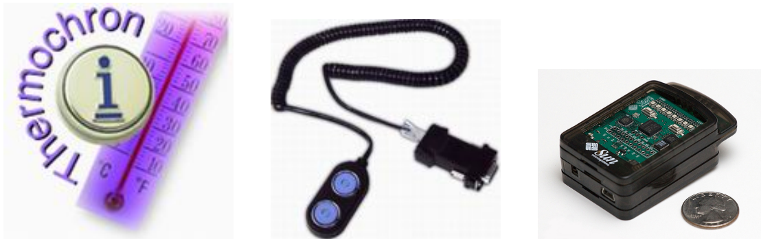
Figure 4.7: Physical Temperature Sensors (iButton, iButton base, SunSpot)
