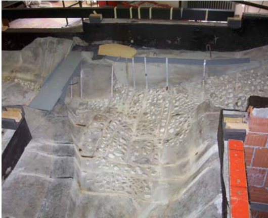
Figure 5.7. Hydraulic Model in non-working conditions
