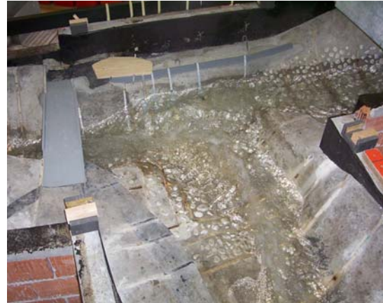
Figure 5.8. Hydraulic Model in working conditions
