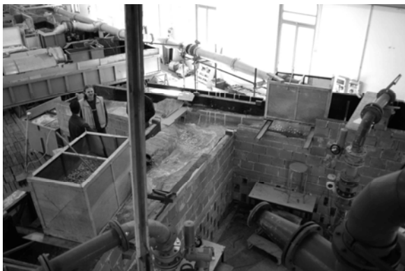
Figure 5.3. A global view of the hydraulic 3D stream confluence model
