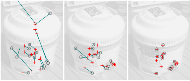
Figure 6: Progression of the recognition loop over a test image at iterations i = \{1, 3, 6\} with N = 16 keypoints. The white circles represent keypoints that are considered as inliers. Red crosses refer to positions that are predicted by the model. Lonely red crosses refers to missing matches caused by occlusion or keypoints detection failure. They are interpolated from the previous ones in a 3D manner. The test image was shot about 45^\circ from the model image’s line of sight, resized smaller and blurred. The final recognition score is about 2.4 on that image.
