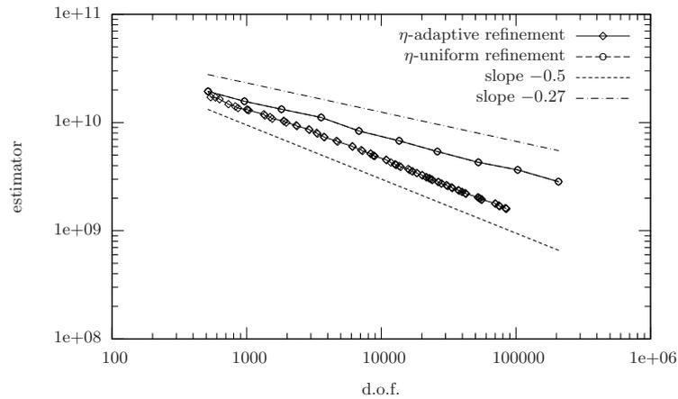
**Fig. 5.7** L-shaped domains: convergence history for  $\eta$  vs. d.o.f., with uniform and adaptively refined meshes.
