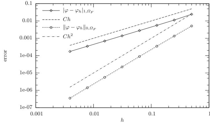
**Fig. 5.3** Problem with analytical solution: convergence history for  $\|\varphi - \varphi_h\|_{0, \Omega_F}$  and  $|\varphi - \varphi_h|_{1, \Omega_F}$ , with uniform meshes.
