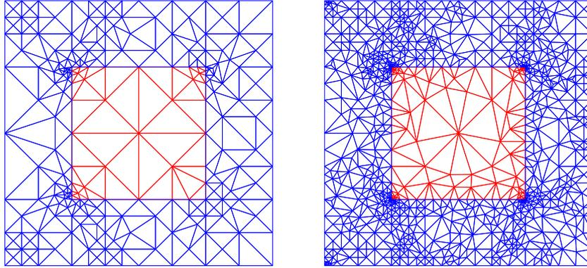
**Fig. 5.9** Incompressible fluid: adapted meshes after 7 (left) and 15 iterations (right).
