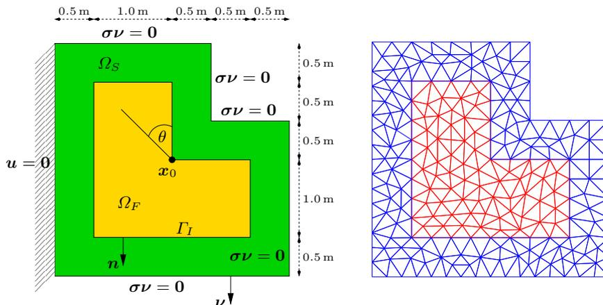
**Fig. 5.5** Sketch of the L-shaped domains (left) and initial mesh (right).
