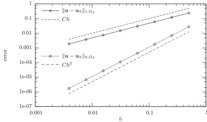
**Fig. 5.2** Problem with analytical solution: convergence history for  $\|u - u_h\|_{0, \Omega_S}$  and  $\|u - u_h\|_{1, \Omega_S}$ , with uniform meshes.
