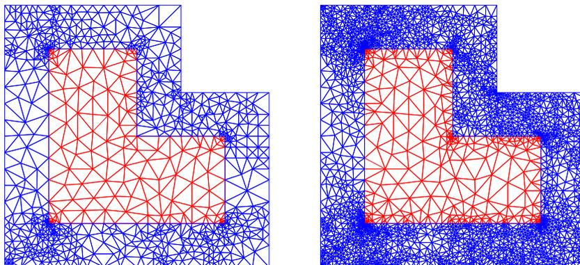
**Fig. 5.6** L-shaped domains: adapted meshes after 15 (left) and 30 iterations (right).
