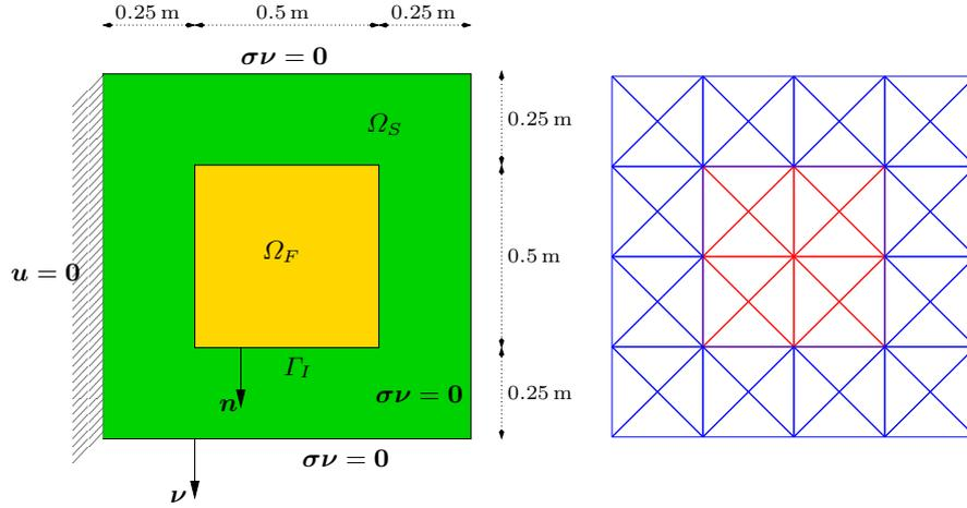
**Fig. 5.8** Incompressible fluid: sketch of the domains (left) and initial mesh (right).
