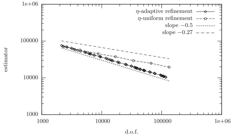
**Fig. 5.10** Incompressible fluid: convergence history for  $\eta$  vs. d.o.f., with uniform and adaptively refined meshes.
