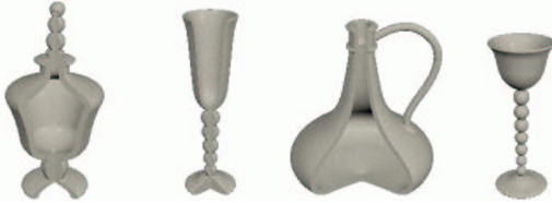
Figure 6: Models created with surface of revolution primitives with varying thickness.
